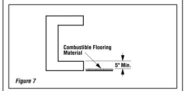
The appliance base may be lower than 5" above the combustible flooring materials if the combustible flooring materials are more than 14" from the fireplace or firebox opening (*Figure 8*).
